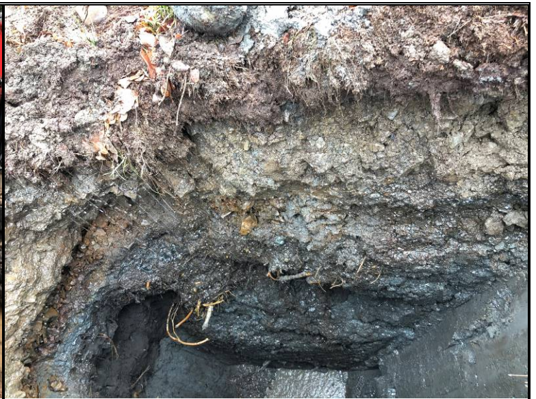
Exposed subsurface soil profile within test-pit TP-1
