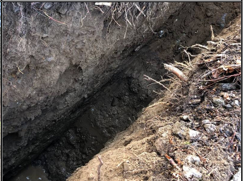
Exposed subsurface soil profile within test-pit TP-8
