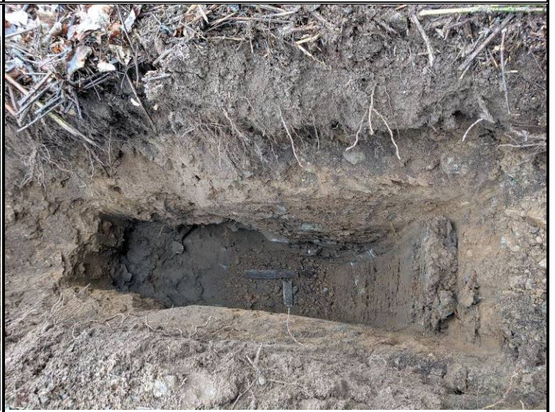
Exposed subsurface soil profile within test-pit TP-2
