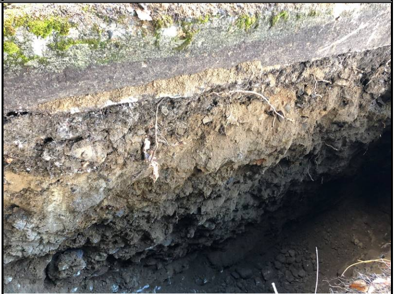
Exposed subsurface soil profile within test-pit TP-6
