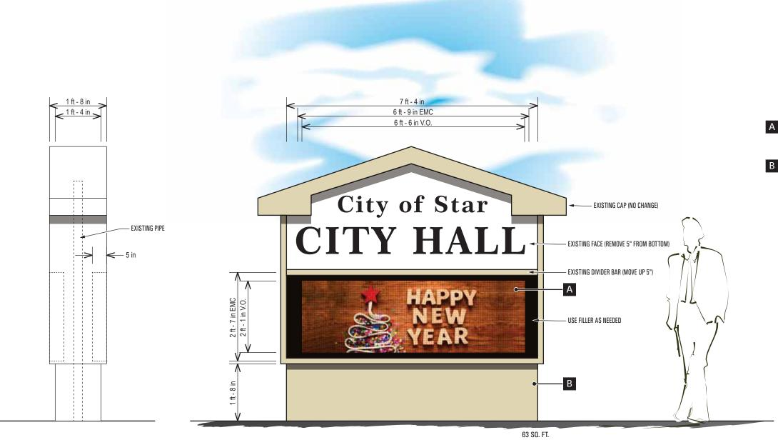
REPLACE READERBOARD W/15.85mm EMC & REPLACE POLE COVER SCALE: ½" = 1'-0" QUANTITY: 1 MANUFACTURE & INSTALL
