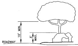
Obstructions between 3' and 10' above the roadway centerline surface elevation are prohibited within sight triangles
