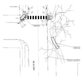
Staff bid a sidewalk connection between the existing sidewalk in Triangle Park and the Able Street sidewalk at Lund Avenue (see diagram to the left) as part of the 2022 Street Improvement project.
