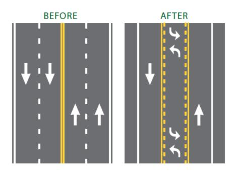
The center turn lane reduces the number of conflict points by removing left turning vehicles from the thru lane. Fewer conflict points along a three-lane section ultimately reduces the total number of crashes and counter rear-end, right angle, and head-on crashes. The Federal Highway Administration cites studies showing a 19 47% reduction in overall crashes when a three-lane
