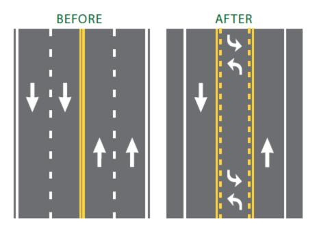
Illustration of the before and after of a four to three-lane conversion or road diet. Image source: FHWA
