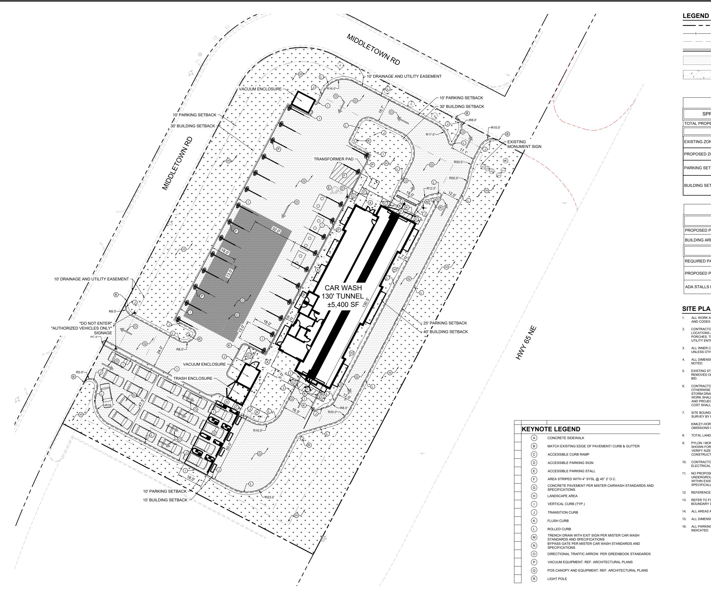
PROPERTY LINE PROPOSED FENCE SETBACK LINE PROPOSED CURB AND GUTTER PROPOSED CONCRETE PAVEMENT PROPOSED CONCRETE SIDEWALK
