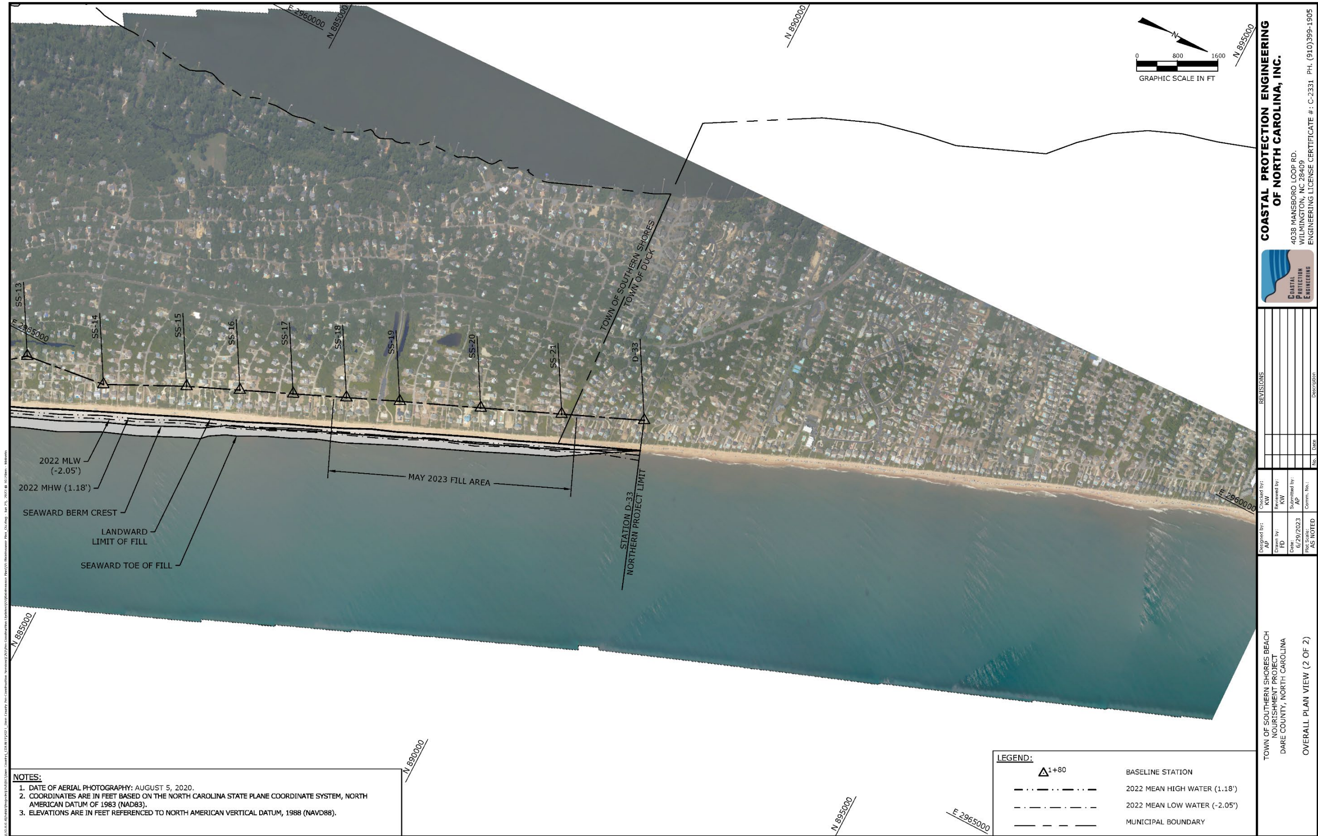
Figure 4. Map showing the extent of the 2022/2023 project including the main fill construction template and the construction baseline (2/2).
