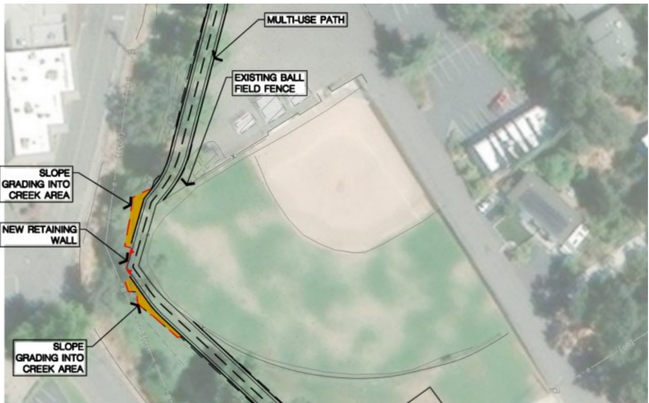
Build Alternative 2: Retaining Wall in Woods Creek
