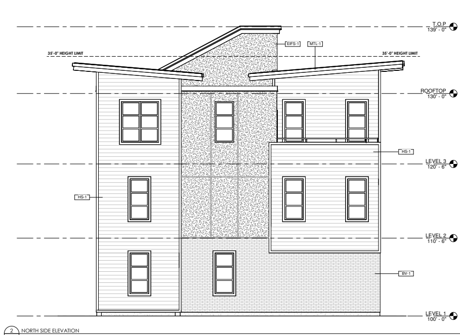
2 NORTH SIDE ELEVATION A201 1/4" = 1'-0"
