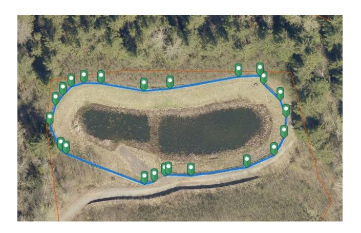
**Swing Pond:** completed 1110 feet of fence to include: Replaced 6 posts and 9 sections of rail, gate post repaired, chainlink stapled.
