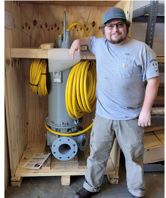
Typical pump (WEMCO) for installation at Kimball Creek Lift Station
