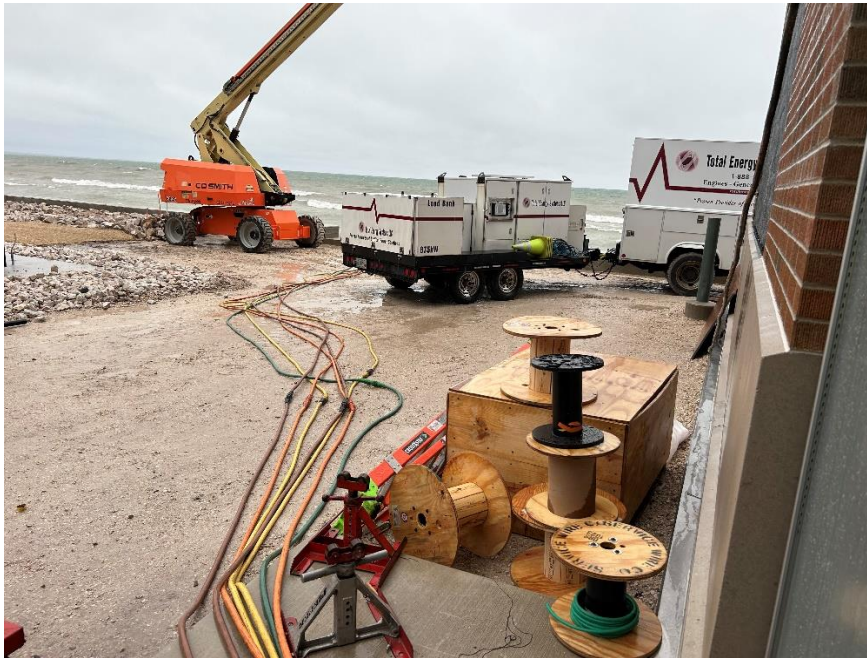
Load bank set up for generator testing.
