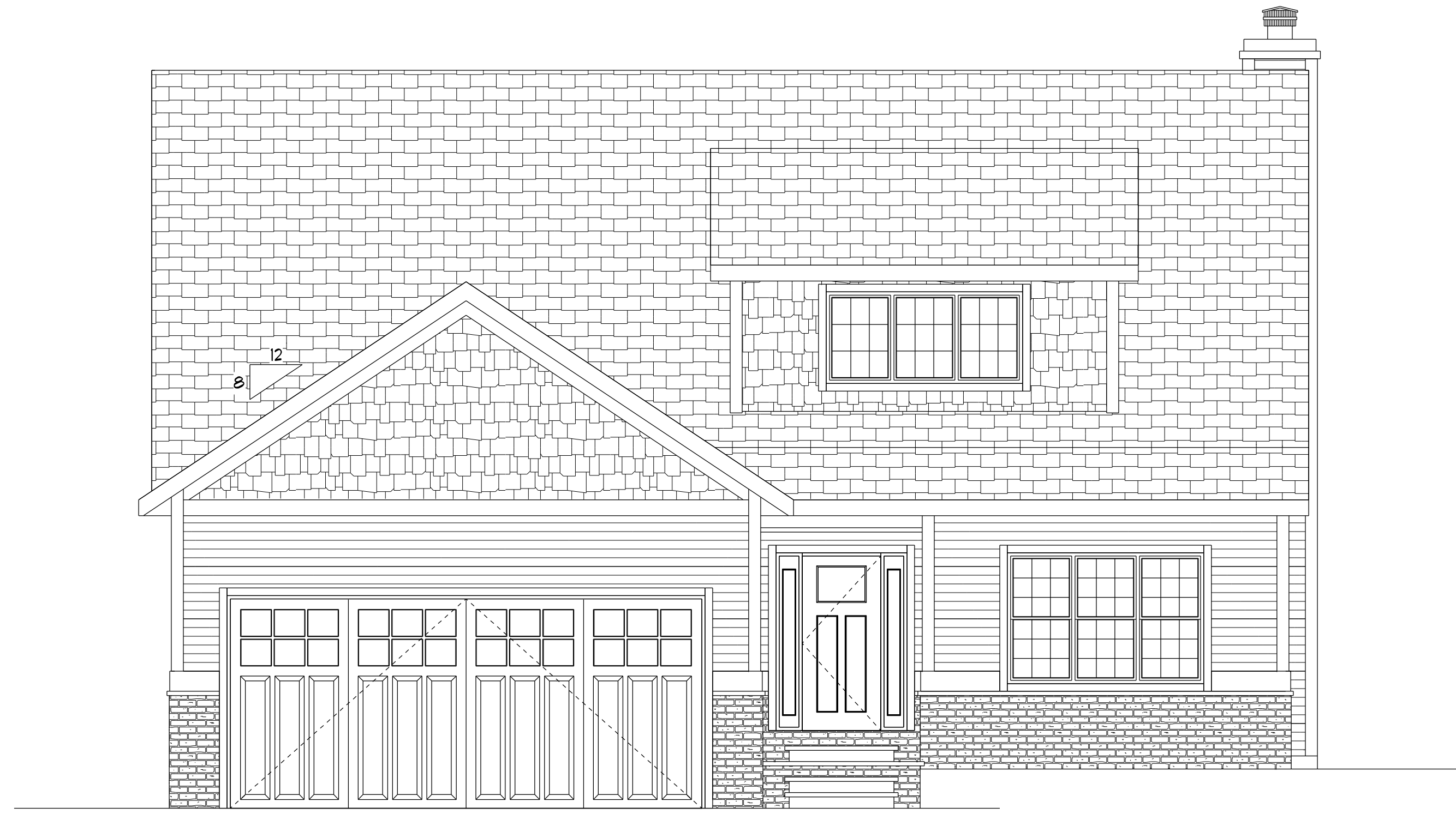
FRONT ELEVATION SCALE: 1/4" = 1'-0"
