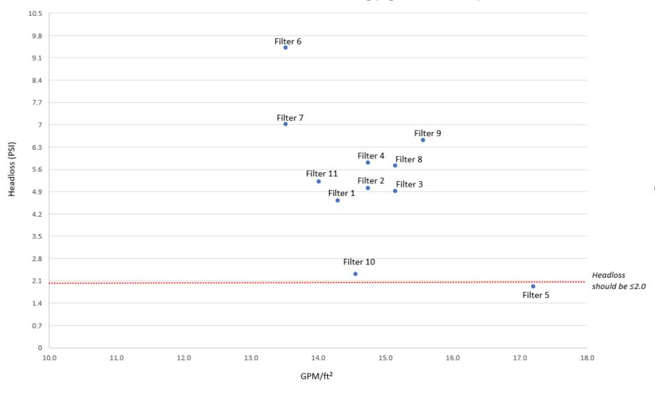
NOTE: 13-15gpm/ft² backwash rate used to minimize over pressurizing Typical backwash rate is 15-20gpm/ft²
