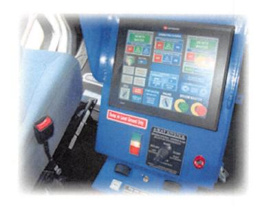
The operator touches LEFT GUTTER BROOM to enable if they want it to run during sweeping operation. Moving the joystick left LEFT GUTTER BROOM will do the same.
