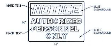
AUTHORIZED PERSONNEL SIGN WHITE/BLUE BACKGROUND, WHITE/BLACK LETTERING MOUNTING LOCATION: GATE & BASE OF TOWER QUANTITY: 1 WHERE ACCESS GATE INSTALLED (QTY: 2)
