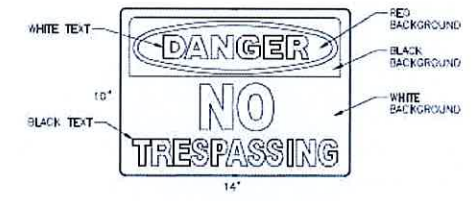
DANGER NO TRESPASSING SIGN WHITE/BLACK BACKGROUND, BLACK/WHITE LETTERING MOUNTING LOCATION: GATE & BASE OF TOWER QUANTITY: 1 WHERE ACCESS GATE INSTALLED (QTY: 2)
