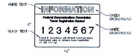
FCC REGISTRATION SIGN WHITE/GREEN BACKGROUND, WHITE/BLACK LETTERING MOUNTING LOCATION: GATE & BASE OF TOWER QUANTITY: 2
