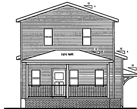
2 PROPOSED SOUTH ELEVATION SCALE 1/8"=1'-0"
