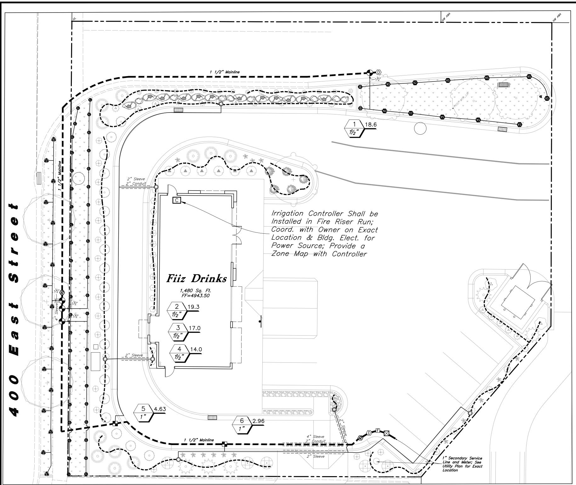
Main Service Line & Other Irrigation Components Are Shown In Paved Or Hardscape Surfaced For Clarity Purposes ONLY! Install All Irrigation Components within Landscaped Areas.
