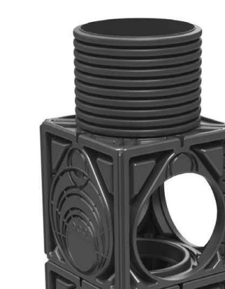
Once the main access chamber has been constructed it will be necessary to add a 18" (450mm) ID raising piece cut to length and placed over the top of the access chamber unit. Once the bases of the upper module(s) have been removed, simply stack units on top of each other ensuring that each module is clipped to the main structure using the StormBrixx® layer connectors.
