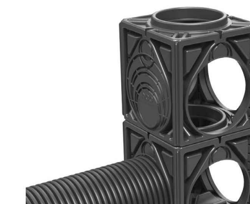
Once the main access chamber has been constructed it will be necessary to add a 18" (450mm) ID raising piece cut to length and placed over the top of the access chamber unit. Once the bases of the upper module(s) have been removed, simply stack units on top of each other ensuring that each module is clipped to the main structure using the StormBrixx® layer connectors.
