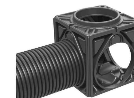
Cut unit as guides for required pipe connection. Push up to 2.5" (65mm) of pipe into access chamber module.
