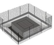
SEDIMENT AND DEBRIS FROM ENTERING THE STORM SEWER SYSTEM; THEREFORE, IT IS NECESSARY TO IMPLEMENT AP AND SEDIMENT CONTROL MEASURES WITHIN INLET DRAINAGE AREAS AS APPROPRIATE.
