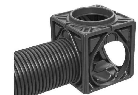
Cut unit at guides for required pipe connection. Push up to 2.5' (65mm) of pipe into access chamber module.
