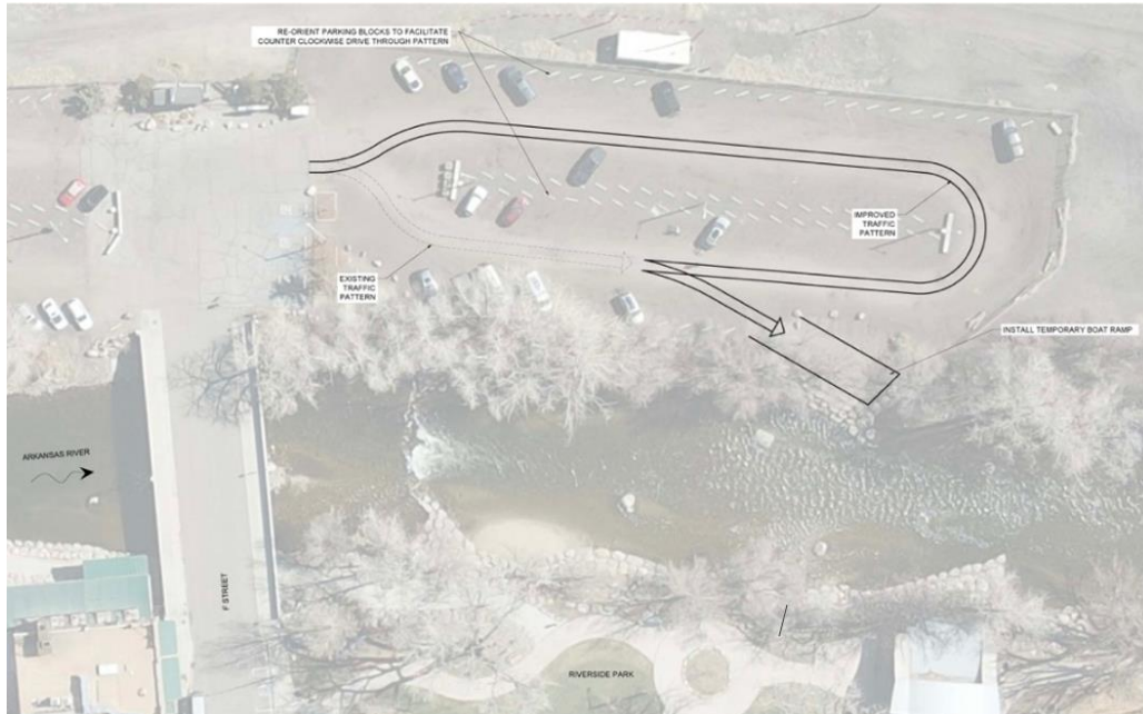
Changed traffic pattern in parking lot to facilitate use of temporary boat ramp. Larger version of this figure located in the Appendix.
