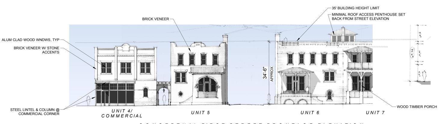
C O N C E P T U A L F I R S T S T R E E T F R O N T A G E E L E V A T I O N
