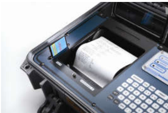
Removable 128 MB CompactFlash™ memory card able to record 10,000 full waveform events.
