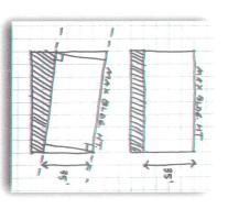
Calculating the cross-sectional area of the parallelogram based on slope:
