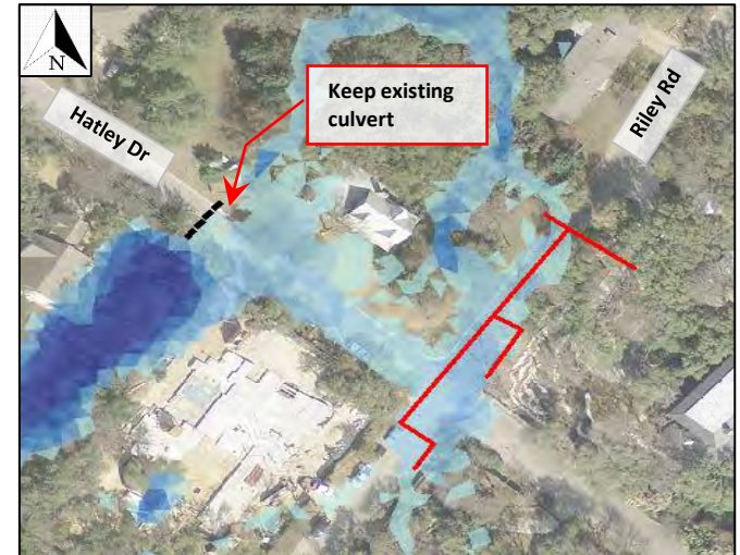
Proposed storm sewer in red. Existing culvert in black. Existing 100-yr inundation shown.
