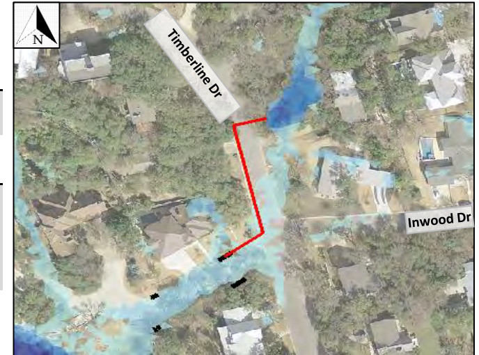
Proposed storm sewer in red to existing inlets in black. Existing 100-yr inundation shown.
