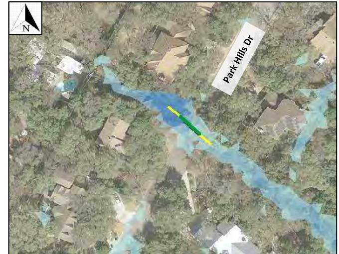
Proposed culvert in green. Channel improvements in yellow. Existing 100-yr inundation shown.
