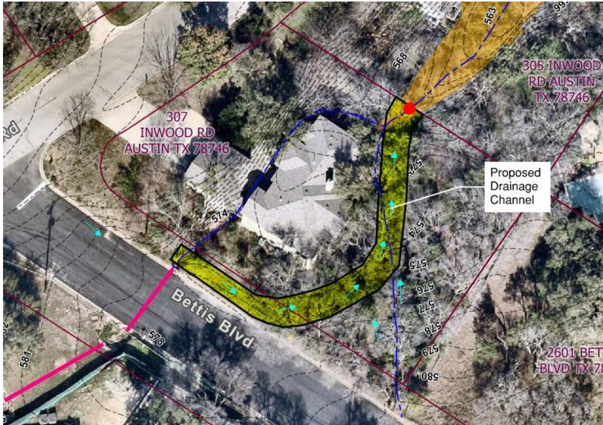
Figure 9 - Option 3 Drainage Channel Concept
