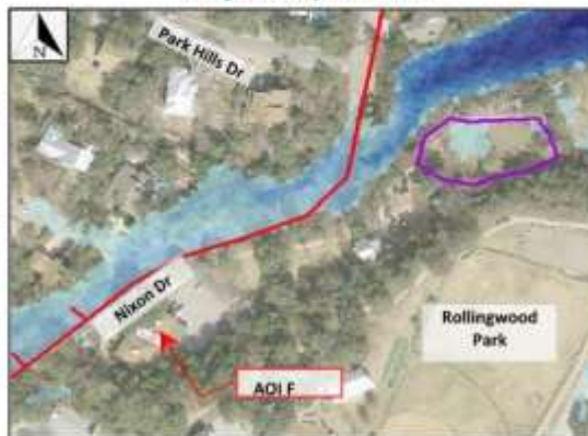
Proposed storm sewer (AOI F) and pond area in purple. Existing 100-yr inundation shown.
