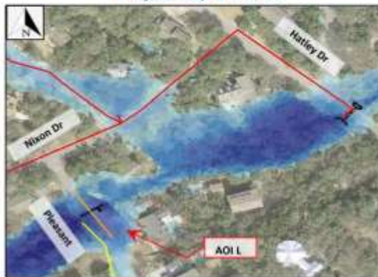
Proposed storm sewer in red. Proposed 12" curb in blue. Existing culvert in black. Existing 100-yr inundation shown.
