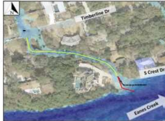
Channel improvements in yellow, proposed storm sewer in red. Existing channel in black. Existing 100-yr inundation shown.
