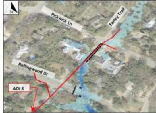
Proposed storm sewer in red, existing in black. Existing culverts in black. Existing 100-yr inundation shown.
