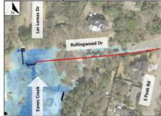
Proposed storm sewer in red. Existing culverts in black. Existing 100-yr inundation shown.
