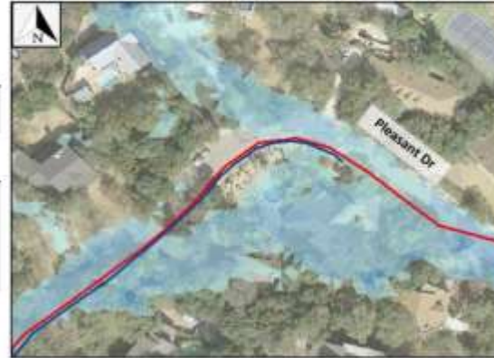
Proposed storm sewer in red. Proposed 12" curb in blue. Existing 100-yr inundation shown.
