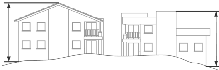
Figure 2-7: Maximum Overall Building Height
