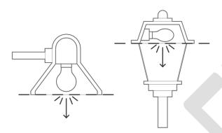
In Figure A (below), the lights on the left are nonconforming. Those on the right can be used in most cases. However, the mounting height and proximity to the property line may cause them to need additional shielding to prevent the luminous elements from being visible from any other property.
