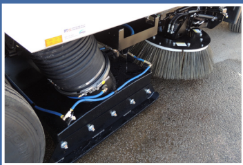
VACUUM AND BRUSH REMOVAL OF DEBRIS
