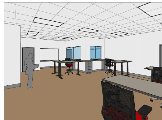
NOTE: BULLET RESISTENT GLASS TO BE PROVIDED AT NEW GLASS. 8' TALL BULLET RESISTANT PANELING TO BE ADDED TO NORTH AND EAST WALL OF RECEPTION AREA
