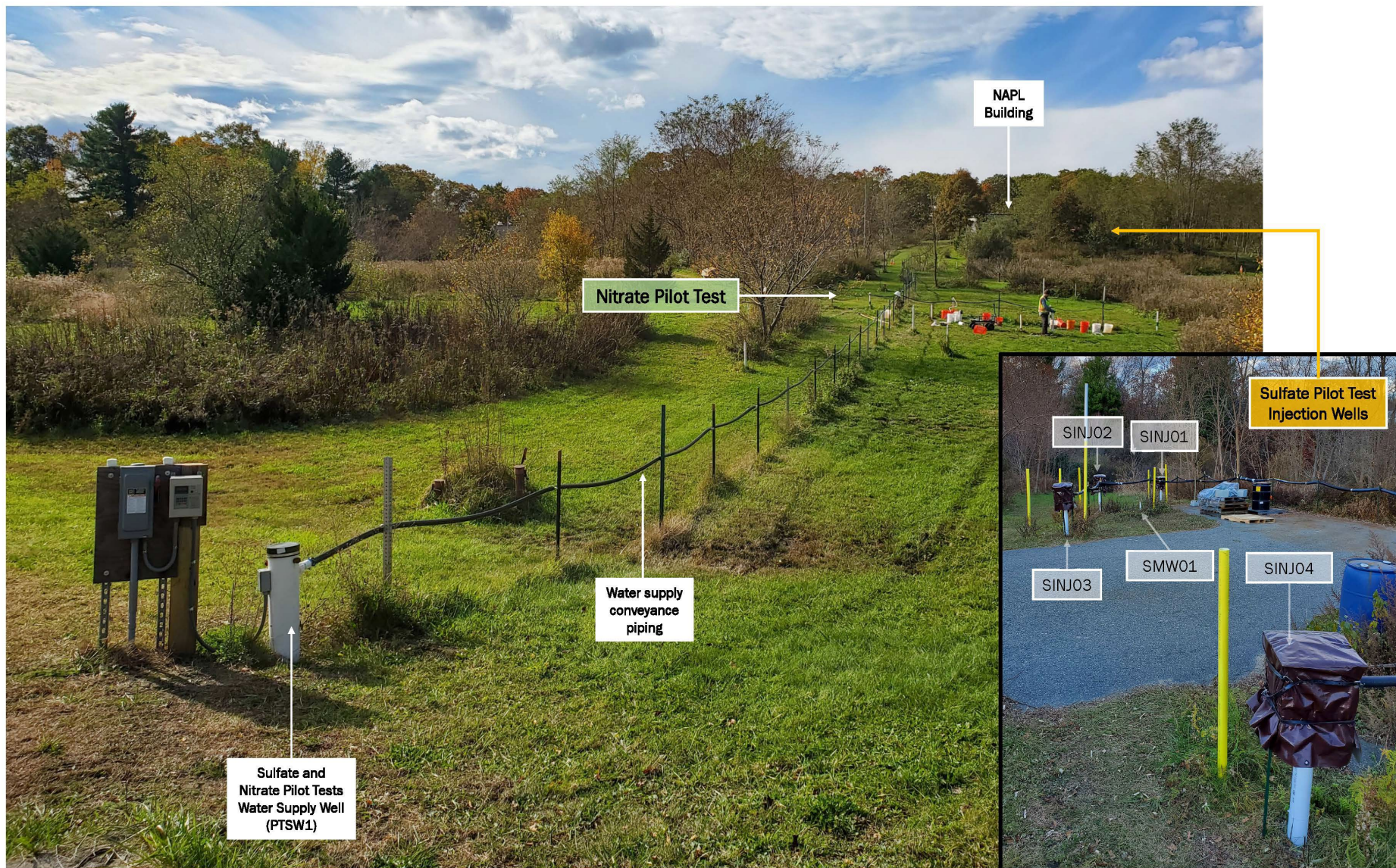
Figure 4.6. Photographs of Sulfate and Nitrate Pilot Test Components Outside NAPL Building
