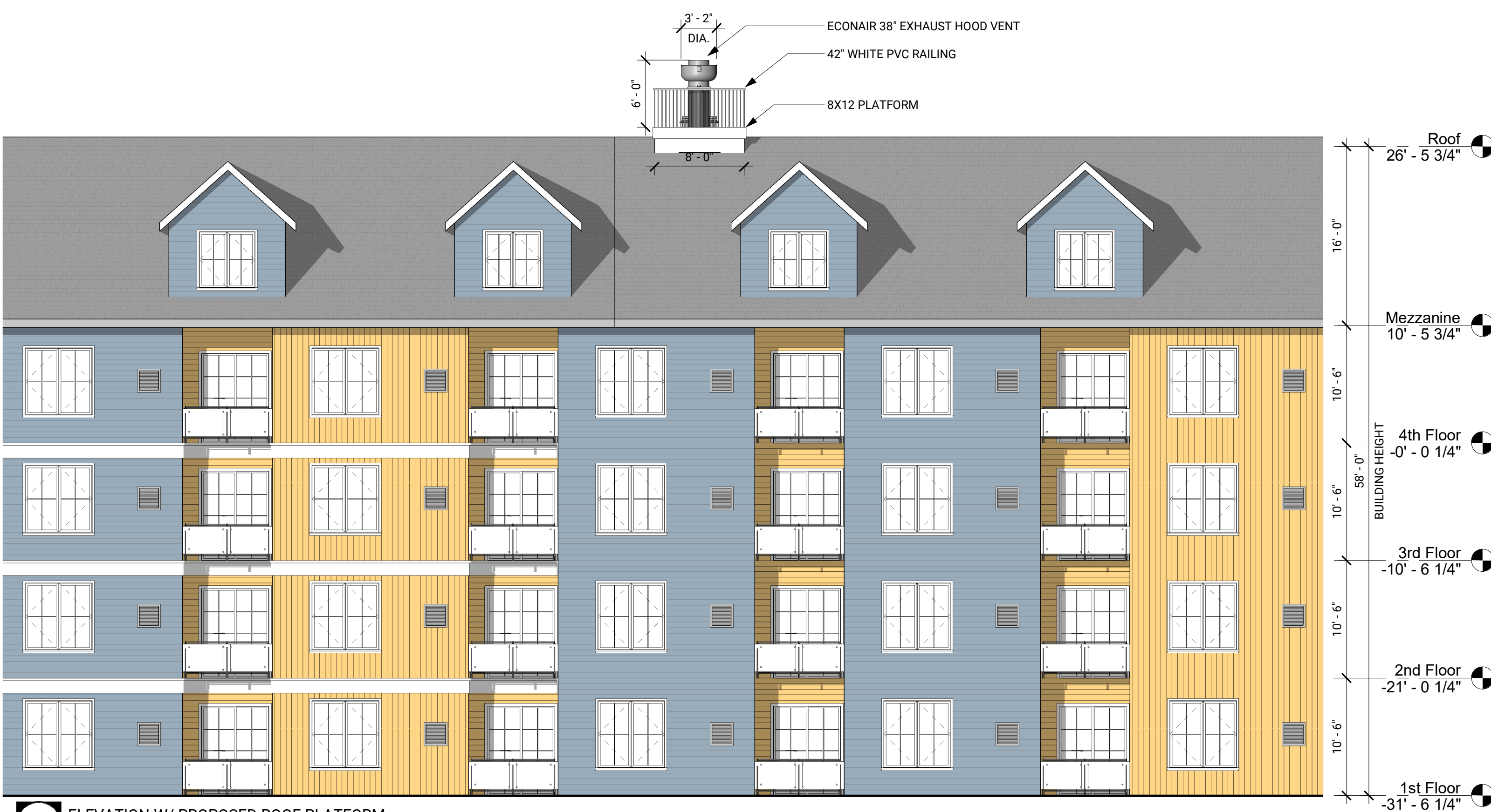
2 ELEVATION W/ PROPOSED ROOF PLATFORM. 1/8" = 1'-0"
