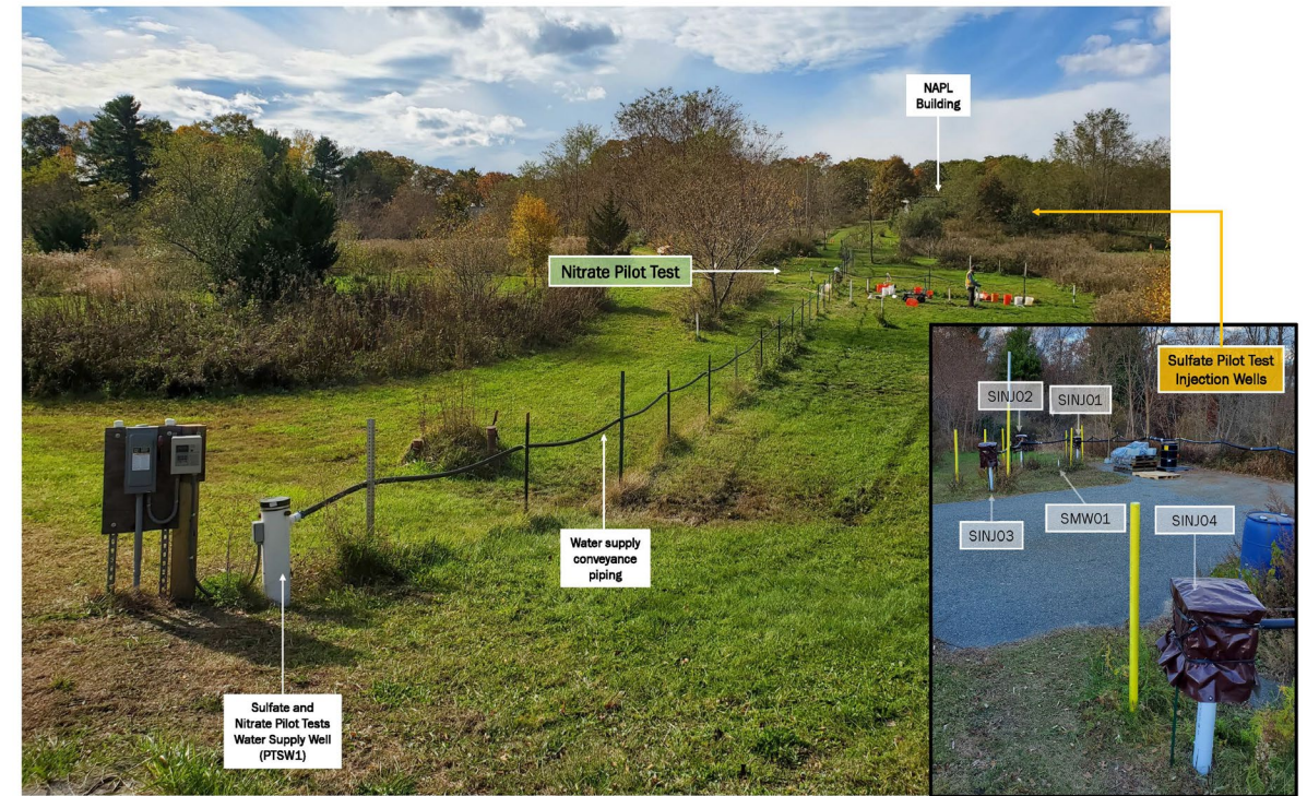
Figure 4.6. Photographs of Sulfate and Nitrate Pilot Test Components Outside NAPL Building
