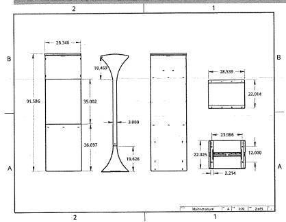
All you need is a 8" long, ½" dia. adhesive anchored on top of threaded rods, min. 4" embedded in concrete. (Proposed Hilti HY 150 Injection Adhesive Anchors). The Soofa Sign is solar-powered and has its own cell service.
