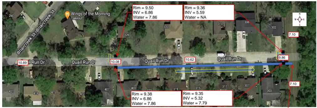
The above illustration shows a layout of the existing storm drainage. Everything flows to the South and to the East as indicated by the arrows. The black boxes represent drain boxes. The gray shaded area represents the area where standing water during rain events in most severe. The yellow shaded area in the illustration to the right represents a section of Quail Run that has been replaced as well as the culverts that connect the drain boxes.
