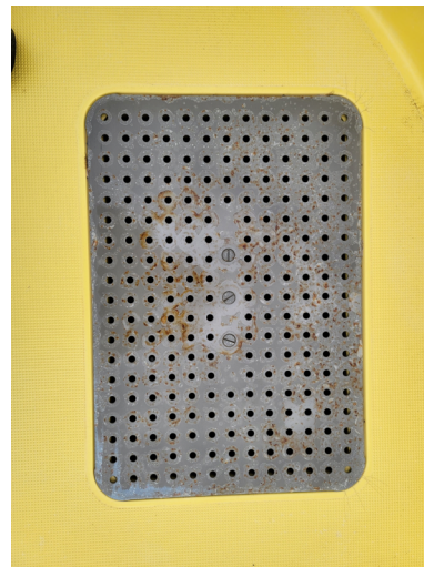
2. CORROSION ON WATER INLET GRATE
