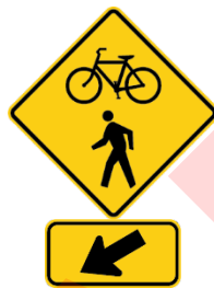
Figure 4-3, Current MUTCD-Standard Trail Crossing Assembly
