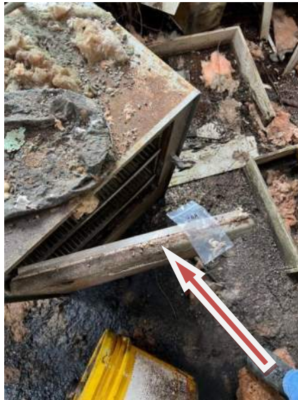
Photograph D-6: Mini-Storage Bldg, Northernmost Rm/lab, white 'rope' packing/gasket around door of old drying oven sitting on floor, contains 55% chrysotile ACM, Category I, non-friable, intact. Pink fiberglass and white ceiling tiles, mostly on floor, do not contain any asbestos.
