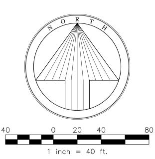
Basis of bearing: State Plane Coordinate System, Texas North Central Zone 4202, North American Datum of 1983. Adjustment Realization 2011.
