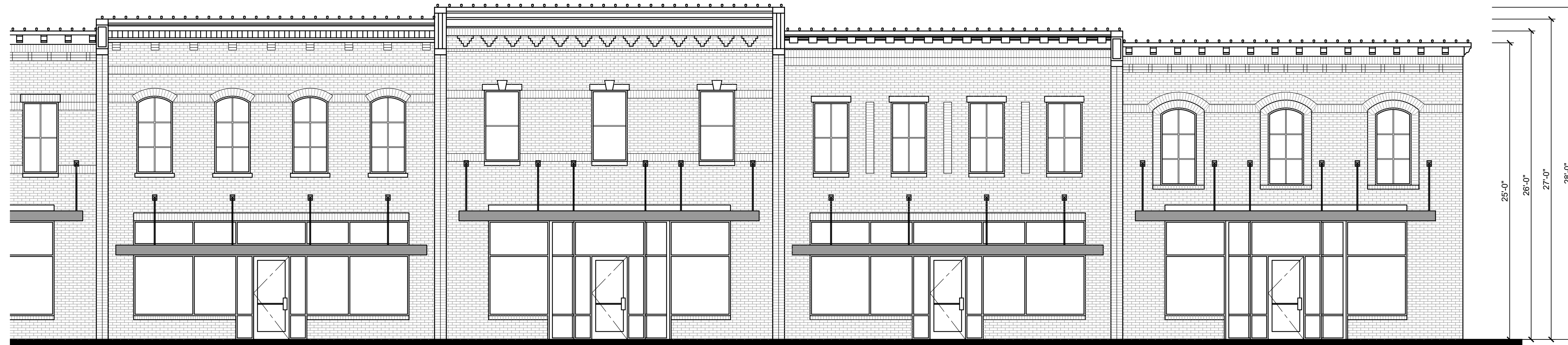
UNIT #11 UNIT #12 UNIT #13 UNIT #14 1 A1.4 3/16"=1'-0" LUXURY OFFICE / WAREHOUSE 11 THRU 14 STREET ELEVATION
