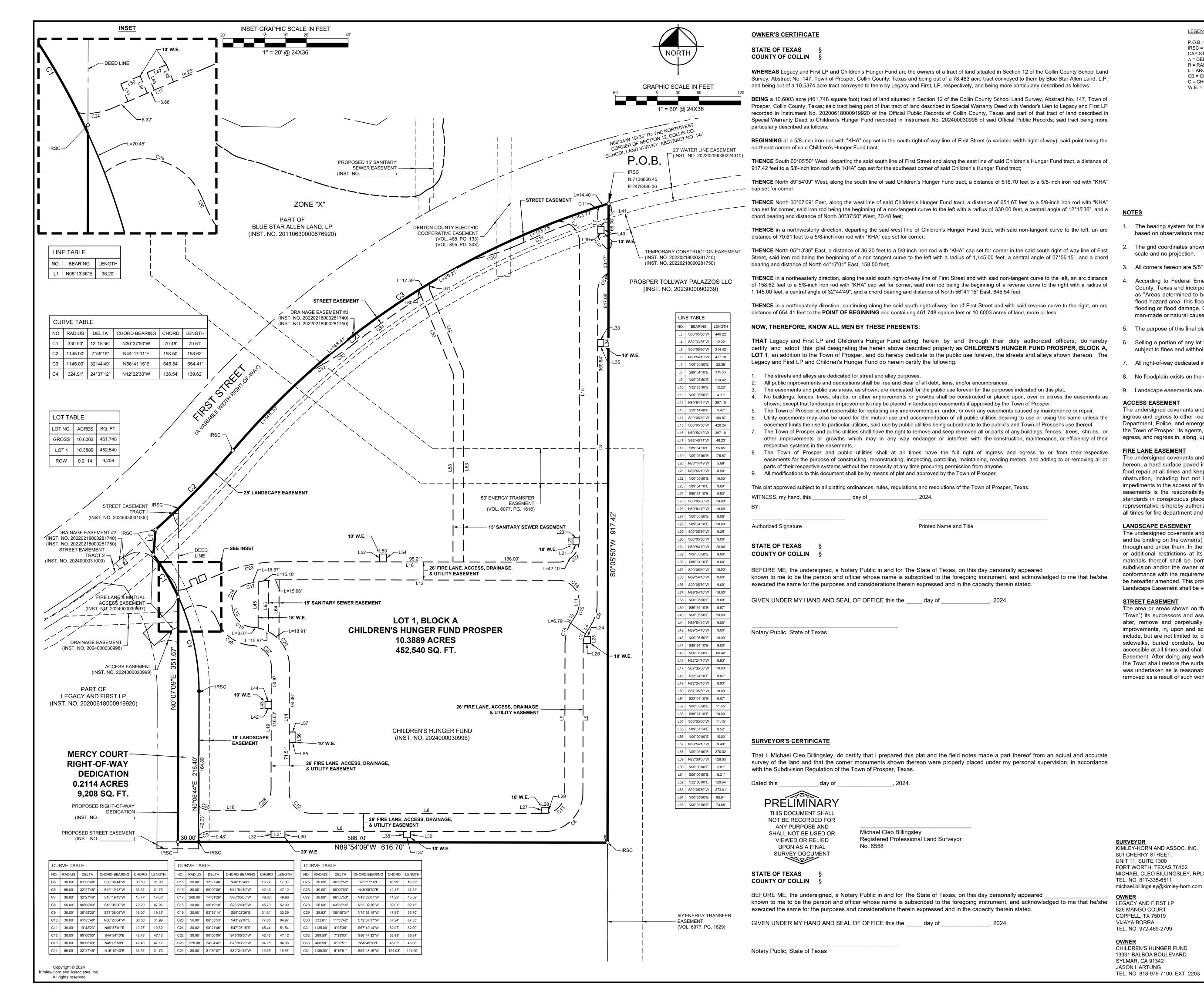
P.O.B. = POINT OF BEGINNING IRSC = 5/8" IRON ROD SET WITH A CAP STAMPED "KHA"  $\Delta = DELTA$ R = RADIUS L = ARC LENGTH CB = CHORD BEARING C = CHORD DISTANCE W.E. = WATER EASEMENT
