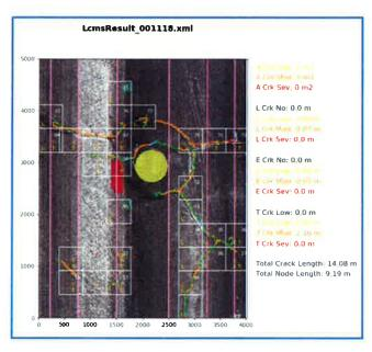
While any engineering firm could deploy the LCMS2 equipment for data collection. processing the information for distress quantification requires а complete understanding of automated technologies, GIS mapping, and distress measurement protocols found in standards such as ASTM D6433. Simply reviewing the LCMS cracking vectors (colored cracks) with the human eye dilutes the objectivity of the equipment.
