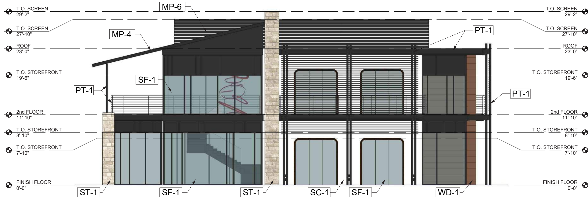
BUILDING 5 - SOUTH ELEVATION 04
