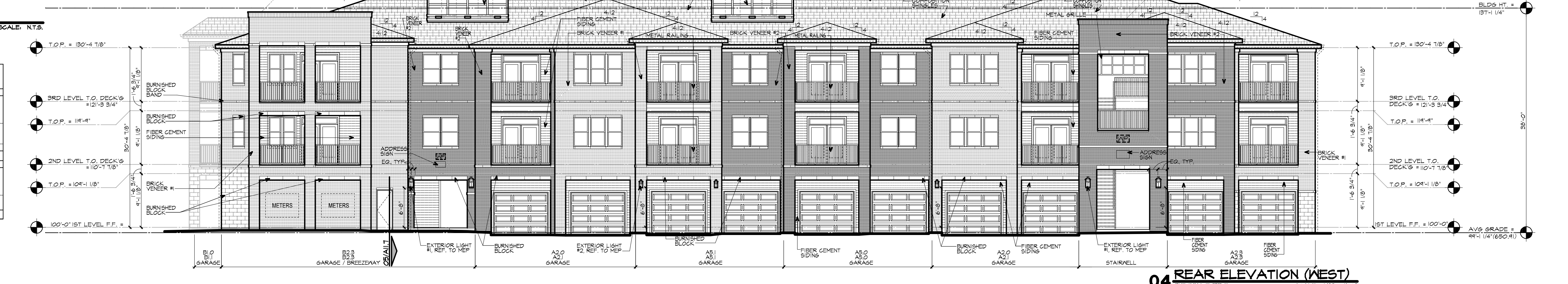
04 REAR ELEVATION (WEST) BUILDING TYPE II SCALE: 1/8" = 1'-0"
