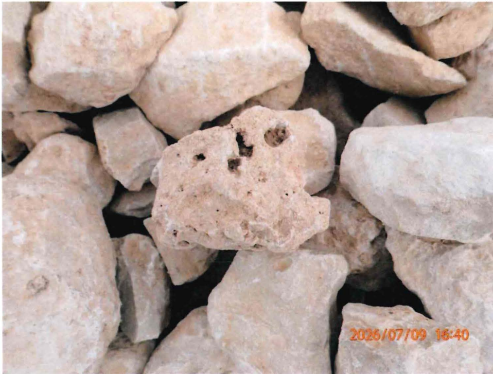
Figure 5. Bedding stone with vugs.
