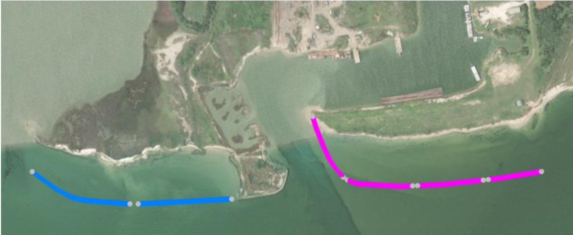
Figure 4.4: Alternative 3A breakwater configuration. Rubble mound breakwater is shown as the magenta line and artificial reef unit breakwater is shown as the blue line.
