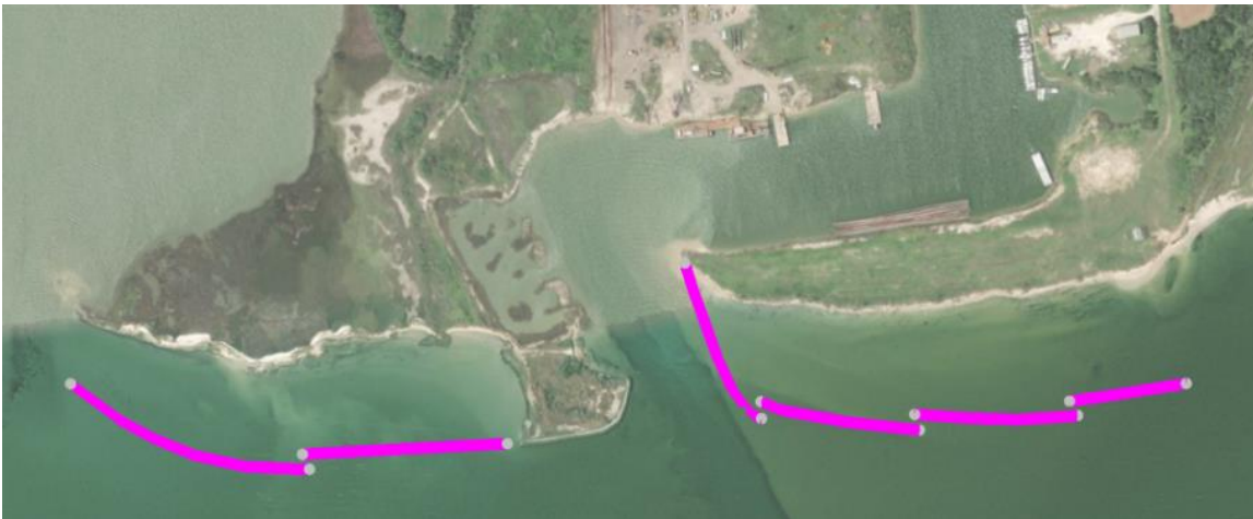
Figure 4.3: Alternative 2 breakwater configuration. Rubble mound breakwater is shown as the magenta line.
