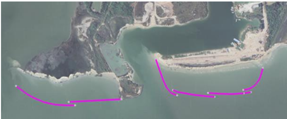
Figure 5.11: Alternative 4A breakwater configuration. Rubble mound breakwater is shown as the magenta line.
