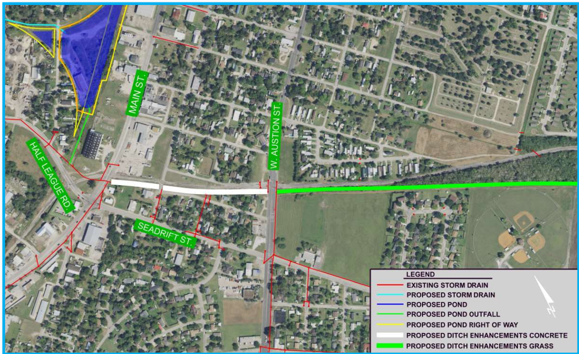
Figure 3.3 Proposed grass/overgrown ditch enhancements.
